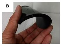
Newly developed EMI shielding caulking material A: Before curing B: After curing
