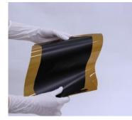
Film covered in a water-based coating using a new SGCNT and shaped into a polyimide sheet
