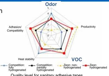
Quality level for sanitary adhesive tapes on a scale where partially hydrogenated resins are 3
