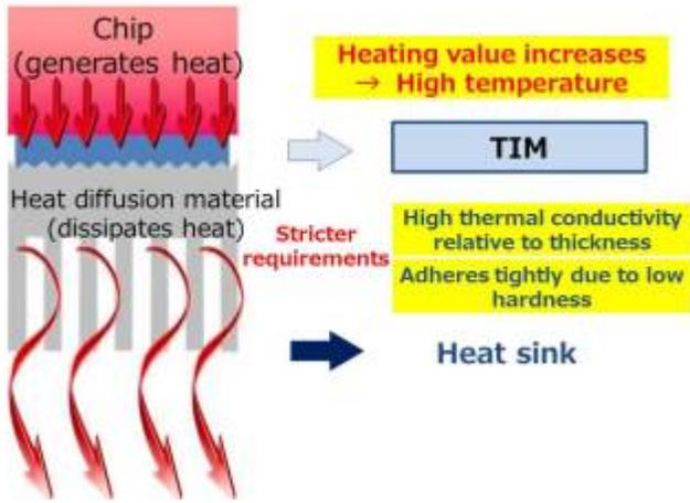
Figure 1 TIM as a Solution for Heat Generation
