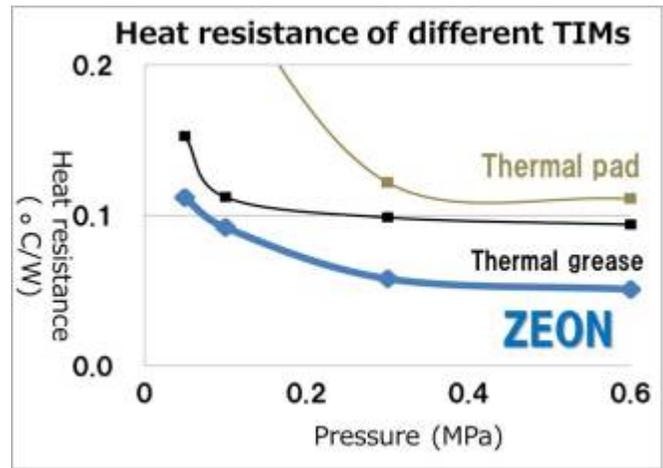
Figure 2 Heat Resistance of New SGCNT Thermal Pad
