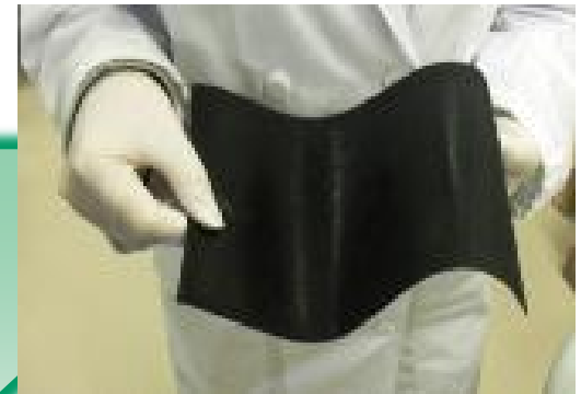
Rubber-CNT composite material
