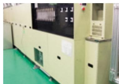
single-walled carbon nanotube large-area continuous chemical vapor deposition synthesis furnace (12m)
