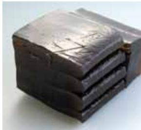
Zetpol® hydrogenated nitrile (HNBR) elastomers
