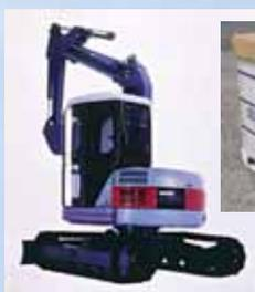
Construction equipment exterior covering made by RIM (Reaction Injection Molding)
