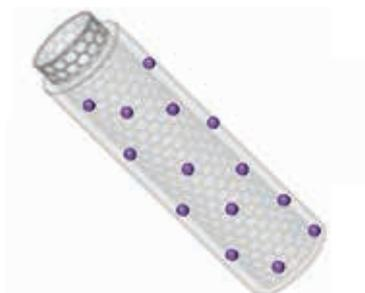
CG image of hybrid catalyst on single-walled CNT
