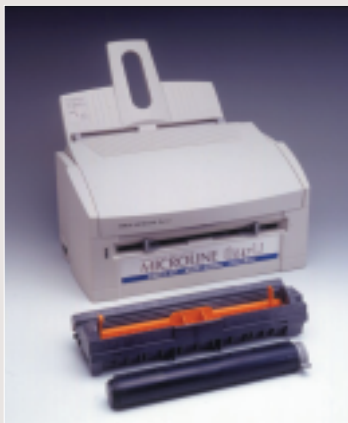
Laser printer using polymerized toner
