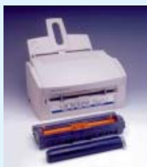
Laser printer using polymerized toner
