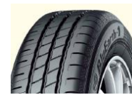
Fuel-efficient tire made with S-SBR
