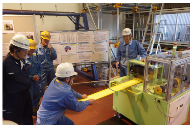
The hands-on safety education covering the dangers of getting caught in a roller
