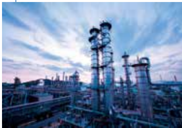
GPB: ZEON process of butadiene. This is a proprietary ZEON technology used to extract highly pure butadiene from C4 fraction.
