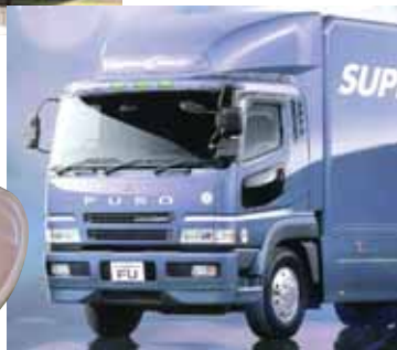
Truck Air Deflectors (Lightweight Structure Improves Vehicle Fuel Economy)
